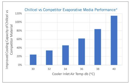
\*Tested in a NATA (National Association of Testing Authorities) accredited laboratory. Cooling capacity calculation based on AS2913, Breezair TBSI580 Cooler and inlet air temperature wb 22°C. Competitor evaporative media saturation efficiency assumed to be 80%.
