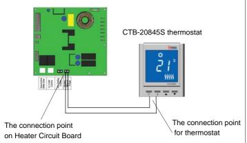
Note: ★ No polarity requirement for the thermostat wiring.
