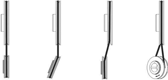
CORRECT ALIGNMENT HORIZONTAL ANGULARITY AXIAL OFFSET VERTICAL ANGULARITY
