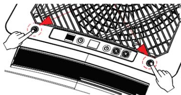
2. Disassemble the grille by pulling down to 45° angle and unclipping from the fascia.
