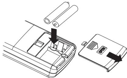
If the remote controller does not activate, remove the batteries and re-insert after waiting 30 seconds.
