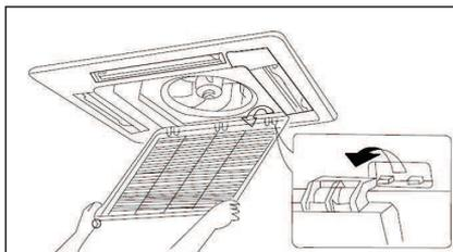
3. Remove the filter mesh. Clean the filter mesh by vacuuming or washing under running water (no warmer than 45°C). Use a mixture of mild detergent and water if the filter has grease or oil buildup. Dry in the shade.
