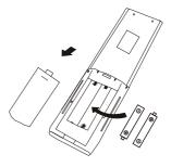
If the remote controller does not activate, remove the batteries and reinsert after waiting 30 seconds.
