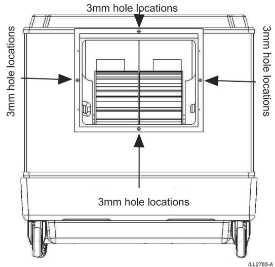
Conduct a test fitment of the grille to the grille frame to check alignment and squareness.
