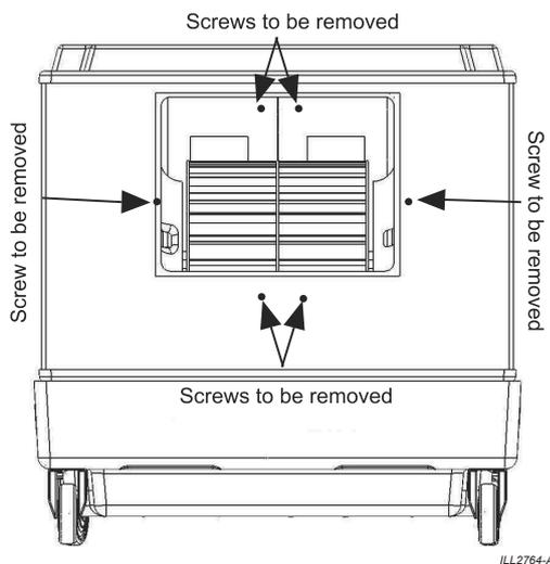
Remove these fasteners and put aside. For those coolers that had previously been used with an integral flexible duct, trim the flexible duct right back as far as it can be trimmed with the sharp knife.
