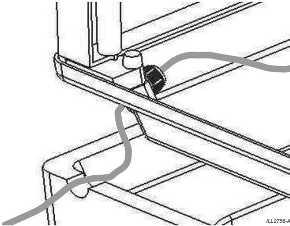
Cut the cable tie temporarily securing the pump (as instructed on Pg 5).
