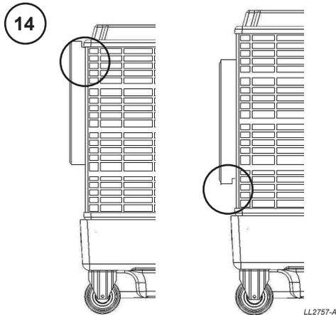
Note the orientation of the notch in the frame of the grille. For small cabinet coolers (EA90) the notch locates under the edge of the lid (Fig. 14 LHS) and for a large cabinet cooler (EA120) the notch is located at the bottom of the frame. (Fig. 14 RHS)
