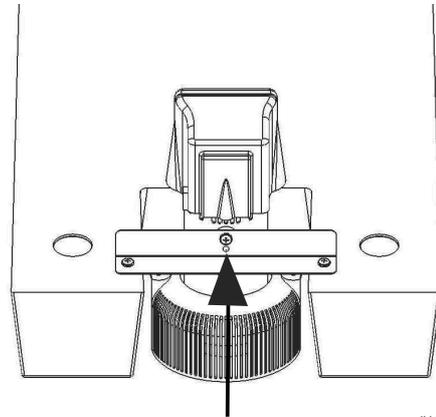
**ENSURE THE FLOATING PLATFORM LOCATES IN PIVOT POINTS IN TANK.**
