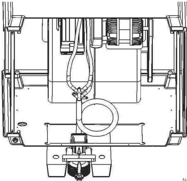
Secure the 4 way connector to the scroll using one of the screws which was previously used to secure the pump to the tank. This will require drilling an appropriate 3mm (1/8") hole in the scroll for the screw if using hand screwdriver. If using a cordless or power driver, a pilot hole may be required.
