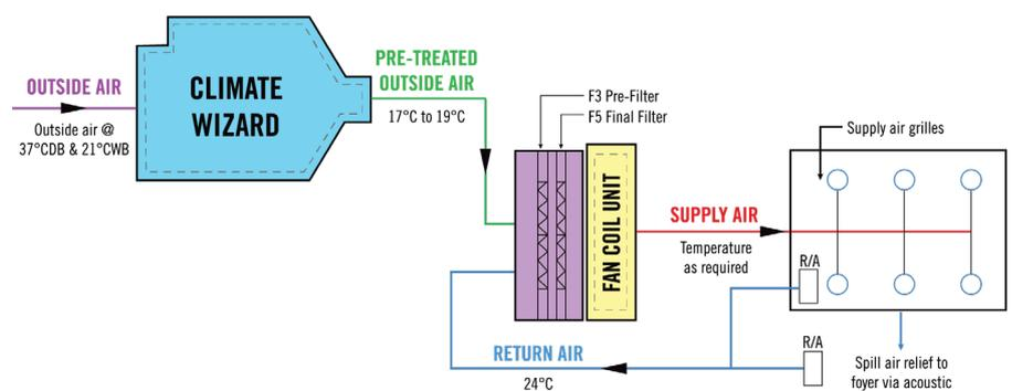
Air schematic for Climate Wizard providing pre-cooling to a fan coil unit in the Palace Nova - Rundle Street cinema complex.
