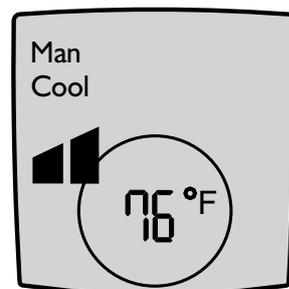
You may then press the "COOL" button to switch between COOL and VENT (VENT = fresh air being delivered but not cooled).
