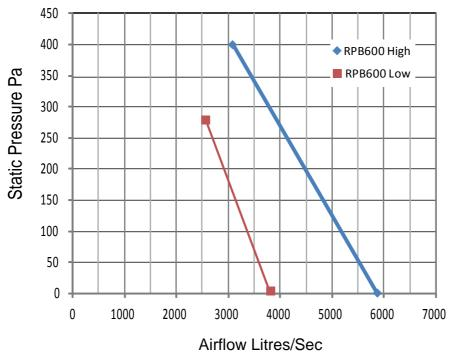
**Note**: Fan curves shown are at constant rated current - free discharge - fixed pulleys. Pulleys for specified pressure applications available on request
