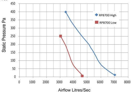
**Note**: Fan curves shown are at constant rated current - free discharge - fixed pulleys. Pulleys for specified pressure applications available on request
