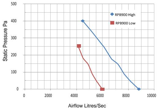
**Note**: Fan curves shown are at constant rated current - free discharge - fixed pulleys. Pulleys for specified pressure applications available on request
