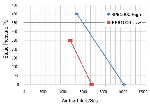
**Note**: Fan curves shown are at constant rated current - free discharge - fixed pulleys.
