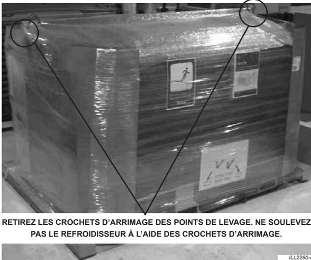
**RETIREZ LES CROCHETS D'ARRIMAGE DES POINTS DE LEVAGE. NE SOULEVEZ PAS LE REFROIDISSEUR À L'AIDE DES CROCHETS D'ARRIMAGE.**
