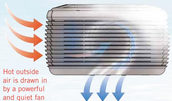
Water absorbs heat by the natural evaporation process. Cool, fresh air is produced
