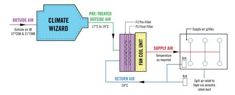
Air schematic for Climate Wizard providing pre-cooling to a fan coil unit in the Palace Nova - Rundle Street cinema complex.
