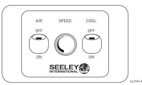
Using the backing plate of the controls as a template, drill 3mm (1/8") fastening holes in the front panel.
