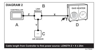
When planning a system installation, consider that the control signal starts from the primary MaglQtouch Controller (A) and travels outwards to each connected component.
