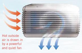
Water absorbs heat by the natural evaporation process. Cool, fresh air is produced
