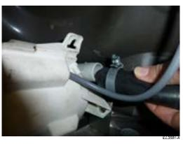
Remove the horizontal rubber hose attached to the circulation pump.
