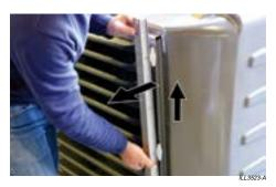
Remove louvre panel by disengaging its bottom clips, and lowering the louvre panel away.
