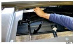
· Lock the handle extension into the front core clamp handle.
