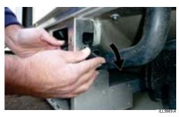
· Pull to remove the solenoid valve from the cooler.
