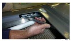
Push down the rear seal clamp handle to engage the clamping of the rear core seals, lock into position with the swinging cam.
