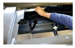
· Disengage the front clamp lever from its clip.
