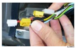
Tape the ends of the cables together making sure the connectors are staggered to form a tapered point.
