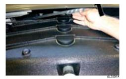
· Disengage the handle extension attached to the rear core clamp from the front clamp lever.
