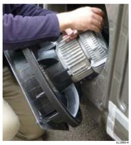
The motor can now be removed from the cooler and replaced. Use a philips head screwdriver.
