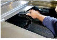
Reach inside the top hatch cover and disengage the swinging cam lock, see below. Pull the rails that seal against the top seal of the cores up towards, away from the cores.
