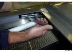
· Using the handle extension, fold the rear clamp handle towards the cooler outlet.
