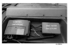
Unplug all wiring and / or pressure tubes required to remove PCBA, unscrew PCBA to remove, carefully noting their positions.
