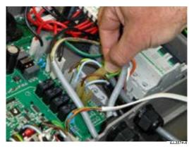
· Unplug the drain pump terminals from the PCBA, noting the position of the wires.
