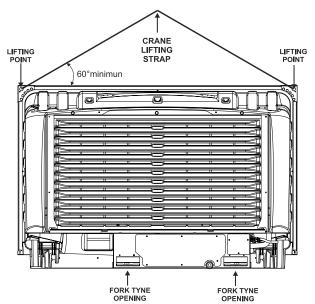
Moving the cooler using Forklift Tyne slot openings.
