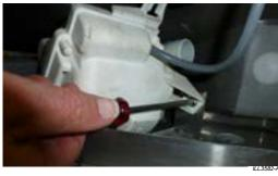
Unscrew the single screw attaching the circulation pump to a tab on the aluminium chassis.
