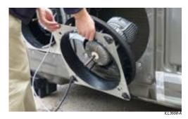
• Thread the connector through the cable gland in the plastic housings. It is recommended that the cable gland inside the cooler is unscrewed from the housing to provide better access when passing the connector through it.
