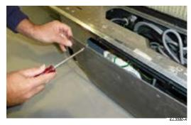
· Remove the pump access cover at the front of the cooler.
