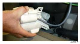
Slide the circulation pump spigot out of the rubber collar in the cooler tank.
