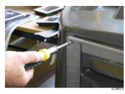
· Un-clip louvre retainers on either side of the louvre panel
