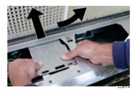
· Slide off the plate that covers the pump by pushing down on the plate to disengage it from a pair of tabs.
