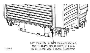
The water supply connection is a 1/2" fitting that connects directly to the internally mounted electric water solenoid valve.
