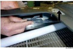
· Swing the front clamp lever towards the cooler outlet.
