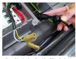
· Remove the cable gland on the side of the electronics enclosure to allow the terminals to be threaded through the gland.
