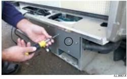
· Rotate the solenoid valve opening/close past the supporting tab, ready to remove it thought the square opening.
