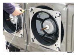
Carefully pull the fan assembly out supporting its weight. It
