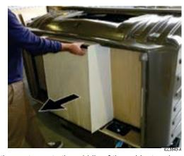
Slide the next core to the middle of the cabinet and remove the spreader, the core can now be removed through the front of the cabinet.
