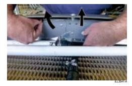
· Reaching in through the top hatch opening, lift the front edge of the spreader and remove from the core.
