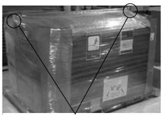
REMOVE TIE DOWN HOOKS AWAY FROM LIFTING POINTS. DO NOT LIFT COOLER USING THE TIE DOWN HOOKS.
