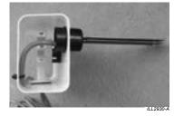
Clean the chlorinator blades by gently wiping the contact surfaces with a soft brush, cloth or non-abrasive wooden or plastic implement. Be sure to clean the inner surfaces of the chlorinator blades. Do not scratch or damage the metallic surfaces of the chlorinator.
