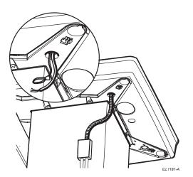
The plug will only insert one way, with the chamfered end first. For now, leave the control cable end in the pan (reservoir) as it will be connected later.
