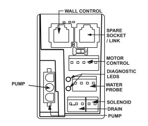
Note! Fit either the shorting plug or water sensor as required.
