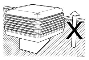
• The cooler must be mounted at least 3m (10') (preferably 5m (17')) away from any TV antenna or antenna cables. Make sure the cooler is not between the antenna and the transmission tower that is providing the television signal to the home.
