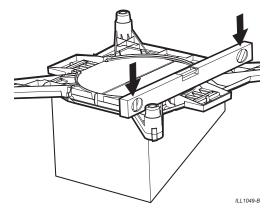
Once level, begin securing the transition to the roof jack using the screws provided. There are eight 'V' notch locations for screws.
