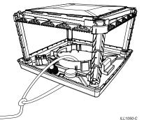
If you intend to pull the cooler onto the roof using a ladder as a slide, then guide the cooler on the underside of the pan (reservoir).
