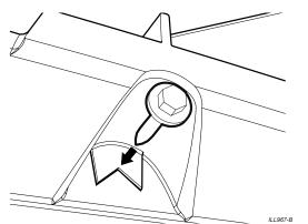
Only use the screws provided. These must be used in the correct positions to prevent interference with the AutoWinterseal. All eight (8) screws must be used. Check the level periodically before driving in all the screws.
