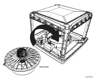
**Important!** Ensure the plug/lead assembly is not caught under the bottom lip of the venturi during installation by holding it out of the way.
