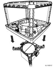
Ensure that the clips in all four corners engage correctly. Do not use any screws to fix the cooler to the transition.
