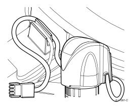
Once the water level is set correctly, isolate the electronics module and connect the pump plug.
