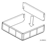
Place the adaptor in the transition and screw in place using the screws provided. Ensure the screws go through both the transition at the eight "V" notch locations and adaptor.
