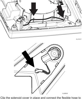
Clip the solenoid cover in place and connect the flexible hose to the mains water supply.
