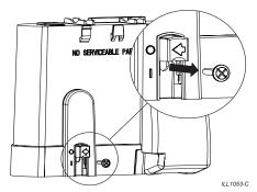
**Note!** Place the electronics module and the screw safely to one side for later use. Do not re-fit the electronics module, as the motor plug will require connection to the underside of the module when the venturi is refitted into the cooler.
