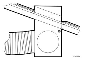
The roof jack may now be flashed to the roof. Make sure there is no chance of water entering the roof space.
