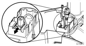
Terminate the power cable in a junction box installed nearby. The fixed wiring must be fitted with an isolation switch that breaks the active (hot) and neutral (common) in accordance with local wiring rules. We recommend the junction box be located and installed on the duct.
