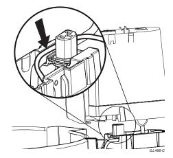
With both cables in place (inside the channel), re-assemble the electronics module and screw it to the pan (reservoir).
