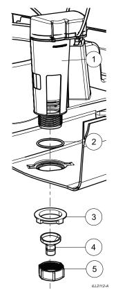
Make sure the "O"-ring (2) is fitted before placing the drain valve into the hole. Screw the nut (3) up tightly by hand underneath to locate the drain valve. Locate the funnel (4) up against the bottom of the drain valve thread and secure with the second, larger nut (5). Make sure that you use the correct drain adaptor. Make sure the drain water discharge flows freely away from the cooler. **Important!** Do not over-tighten plastic fittings.
