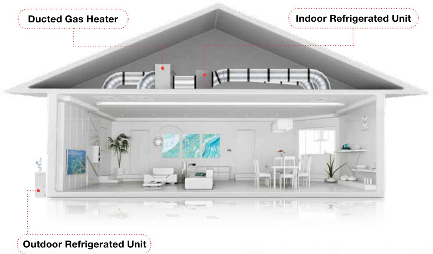
2. Applicable to installations where airflow requirements and duct design are suitable. Not all models of Braemar ducted gas heaters are suitable for add-on cooling, so please check with the dealer.
